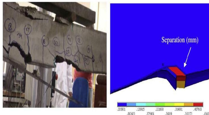
**Fig 9 Simulated and Experimental Results of CFRP Plate De-Bonding**
